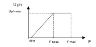
In analog mode, the control frequency of the converter is directed by entry 0 - 10V FREQ.
